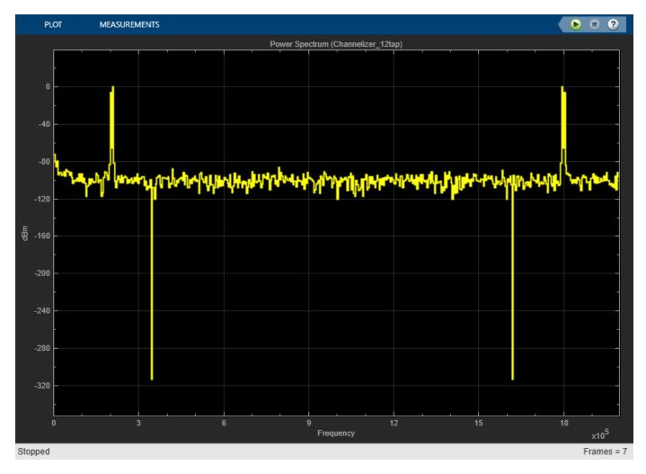
The spectrum viewer shows that the 12-tap filter separates the spectrum of the two signals. Zoom in between 100 kHz and 300 kHz to see where the channelizer detects two peaks. Two peaks is the expected result because the input signal has two frequency components.
