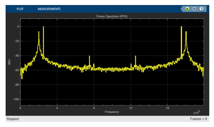
The polyphase filter bank spectrum viewer shows the improvement in the power spectrum and minimization of frequency leakage and scalloping compared with using only an FFT. By comparing the two spectrums, and zooming in between 100 kHz and 300 kHz, you can see that the polyphase filter bank has fewer peaks over -40 dB than the classic FFT.
