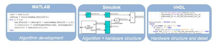
While both MATLAB and Simulink support automatic generation of HDL code, you must construct your design with hardware requirements in mind, and Simulink is better-suited for cycle-based
