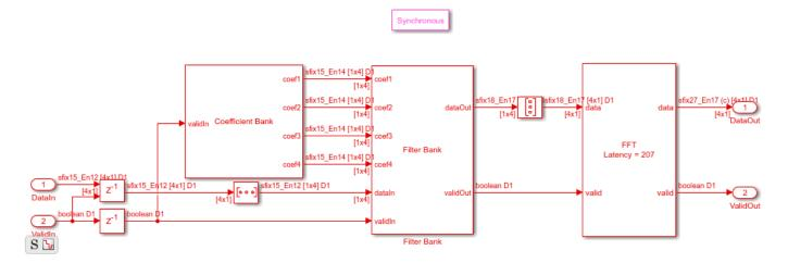
This model diagram shows the pipelined 4-tap filter implementation.
